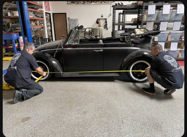
Squaring rear to front — the alignment most VWs never got.
